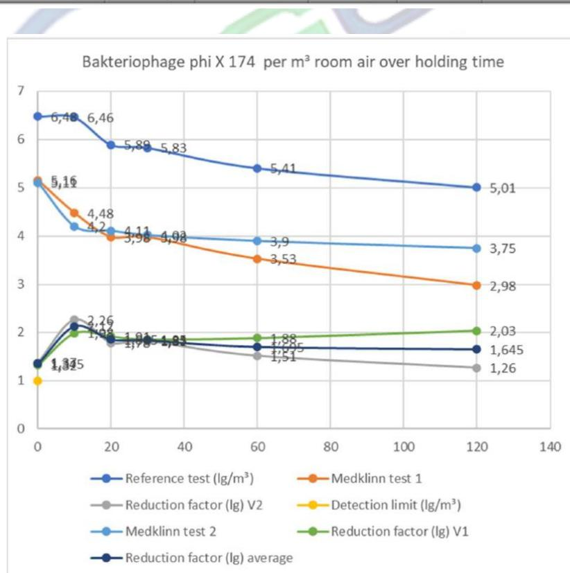
After 10min the maximum reduction factor was measured as a 2.12lg reduction (99% reduction) compared to the reference test, when the Medklinn PRO AS2 Air+Surface
